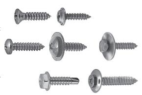
**Teks**<sup>®</sup>: A screw with a drill point that drills its own hole as it is installed. Most Auveco Teks<sup>®</sup> screws have a #2 point which is recommended for material up to .110" thick. The higher the drill point number, the thicker that material it can drill though. Once the metal is penetrated, the Teks<sup>®</sup> fastener functions as a conventional tapping screws.
