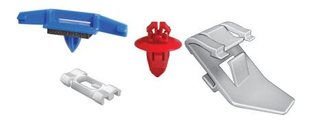
**Nylon Nuts:** Used with metal tapping screws throughout the car (interior & exterior) for attachment. As a tapping screw is installed, it cuts its own thread and spreads the bottom part of the nut apart thus securing it in place. Nylon nuts can be found in door panels, headlight/front-end applications, license plate brackets, arm rests, instrument panels and many other areas. Example: 11719, 13932
